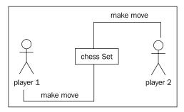
What is that? It doesn't quite look like our earlier class diagrams. That's because it isn't a class diagram! This is an **object diagram**, also called an instance diagram. It describes the system at a specific state in time, and is describing specific instances of objects, not the interaction between classes. Remember, both players are members of the same class, so the class diagram looks a little different:
