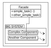
Facade is, in many ways, like adapter. The primary difference is that the facade is trying to abstract a simpler interface out of a complex system; the adapter is only trying to map one existing interface to another.
