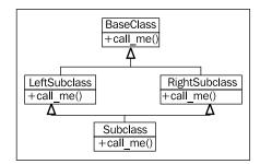
Diamonds are what makes multiple inheritance tricky. Technically, all multiple inheritance in Python 3 is diamond inheritance, because all classes inherit from object. The previous diagram, using object.\_\_init\_\_ is also such a diamond.
