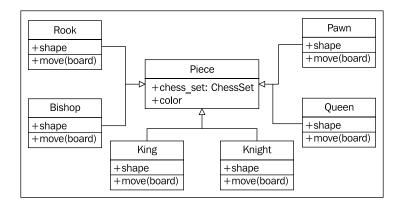
The hollow arrows, of course, indicate that the individual classes of pieces inherit from the **Piece** class. All the subtypes automatically have a **chess\_set** and **color** attribute inherited from the base class. Each piece provides a different shape property (to be drawn on the screen when rendering the board), and a different **move** method to move the piece to a new position on the board at each turn.
